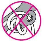
Special care should be exercised with the power cord during steam cleaner use as excessive twisting and/or subjecting it to a substantial external shock can result in damage, which can in turn cause product malfunction.
